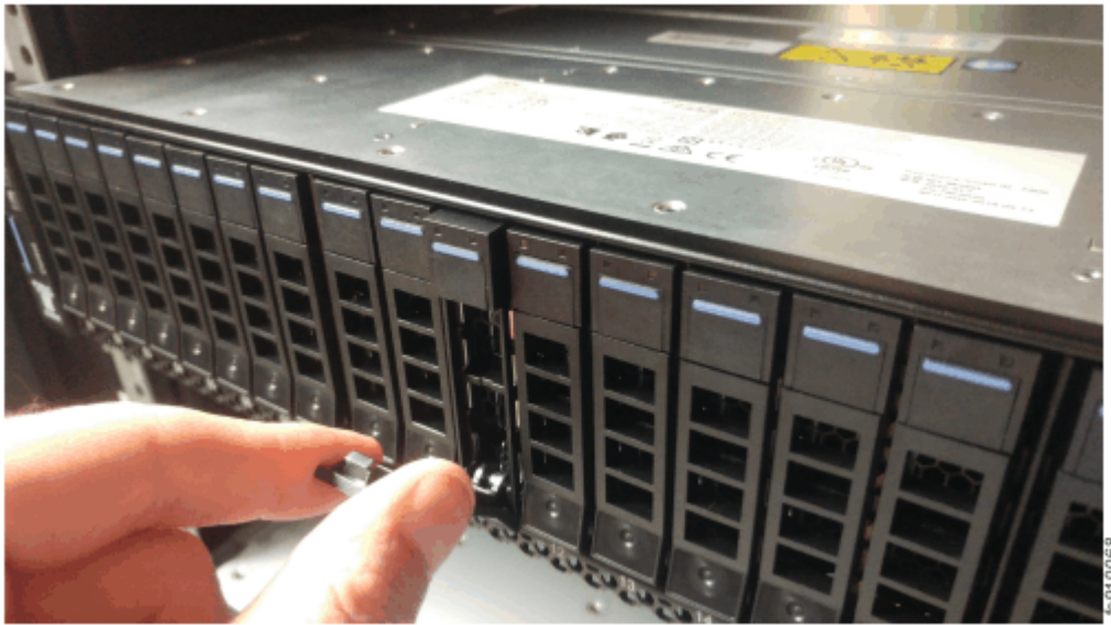
Figure 3. Inserting the new drive
