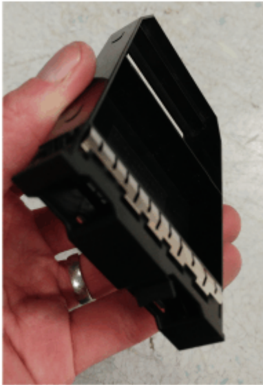
Figure 5. Correct drive blank orientation
