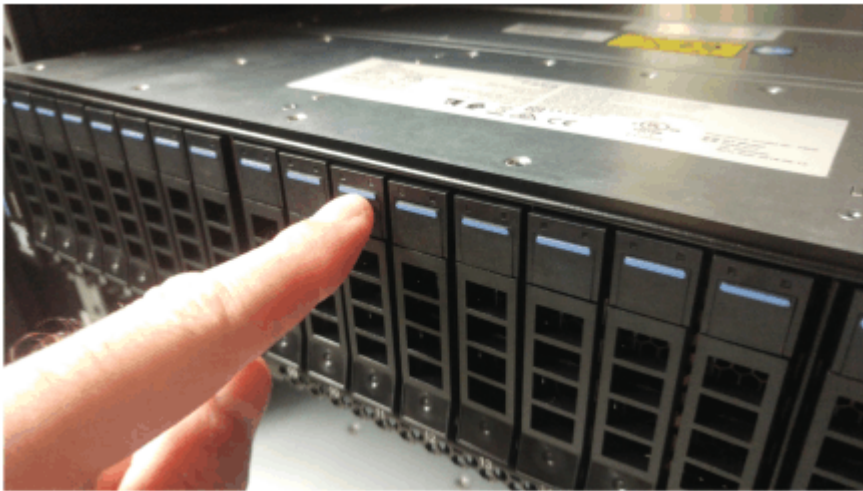
Figure 1. Unlocking the drive and release latch
