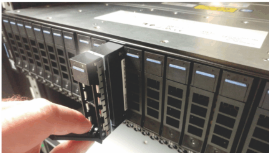
Figure 2. Removing the drive
