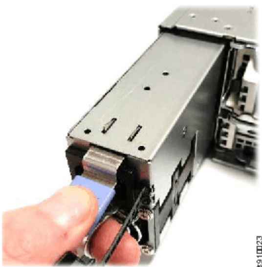
Figure 8. Removing the power supply unit
