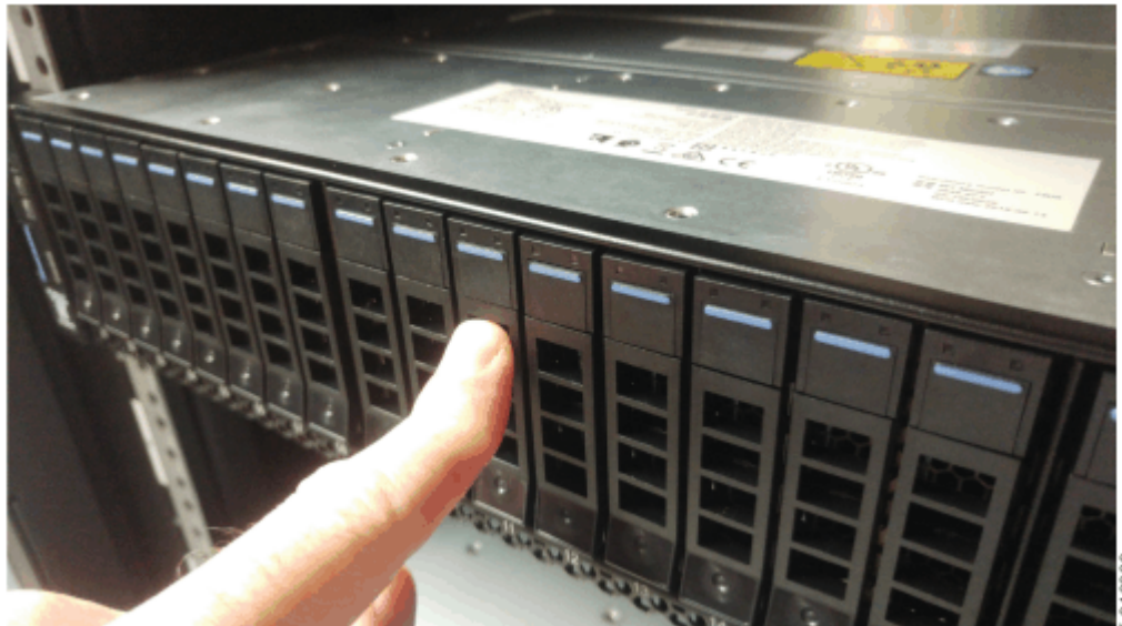
Figure 4. Completing the drive installation
